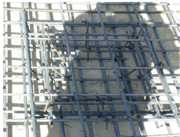
Figure 4: Steel cage used in the second specimen, PSW8-8, showing the swimmer bars.
